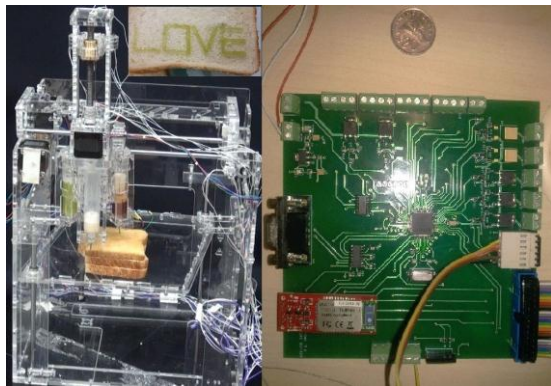
Fig. 6 (Left) FoodieFab mechanism with example output (Right) Design of master board
